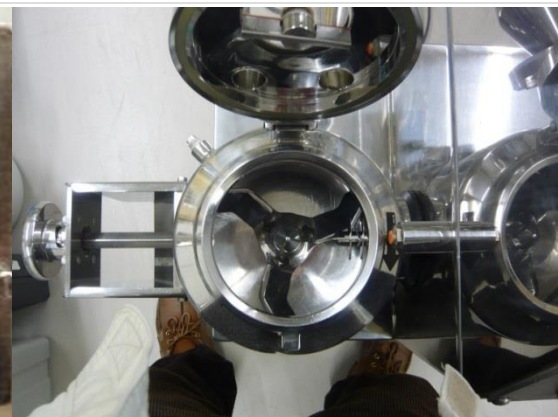
Two kinds of agitating wet granulator
