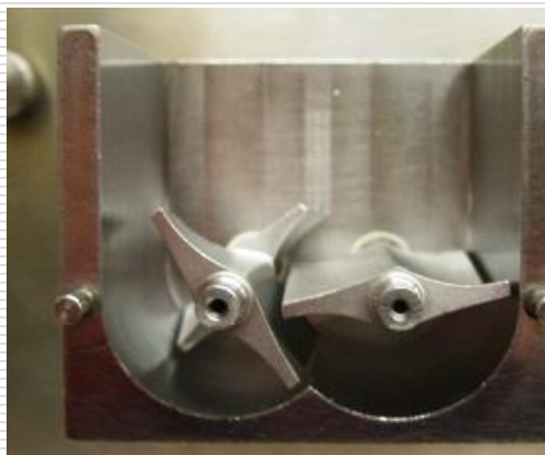
Two kinds of agitating wet granulator
